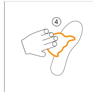
4. Clean the bottom side and the top side of sensor insole with damp soft wipe, then dry with a clean soft wipe
