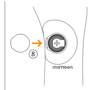
8. Attach battery lid to sensor insole
