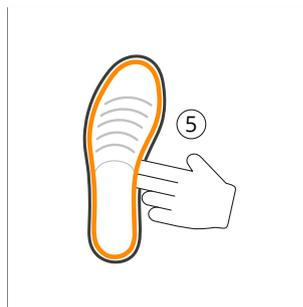
5. To remove the sensor insole, slightly lift sensor insole in medial mid foot area with fingers
