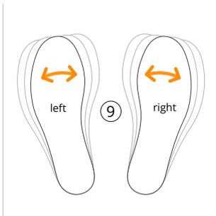
9. Shake left and right sensor insole 2-3 seconds to activate them (auto turn on/off, no switches)
