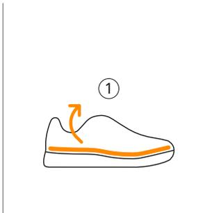
1. If the shoe has a removable inlay or liner, remove it before inserting the sensor insole.
