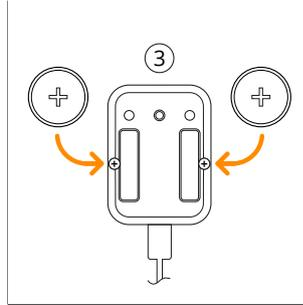
3. Insert coin cell batteries in charging slots, "+" terminal outwards
