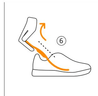
6. Pull on the heel area to remove sensor insole from shoe, do not bend in mid foot area
