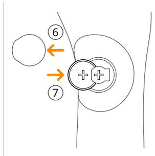
6. Remove battery lid from sensor insole
