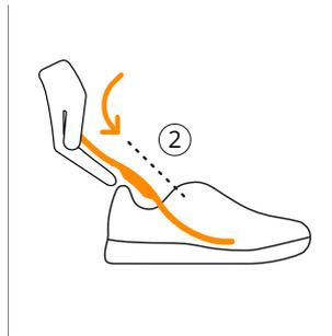
2. When sliding the sensor insole into the shoe, pay attention not to bend the mid foot area
