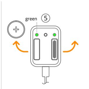
5. Green lights indicate full charge status, remove coin cell batteries from charging slots
