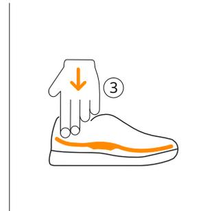
3. Push heel area down to ensure sensor insole sits completely in the shoe
