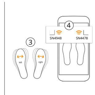
3. For sensor insole interaction shake 2-3 seconds
